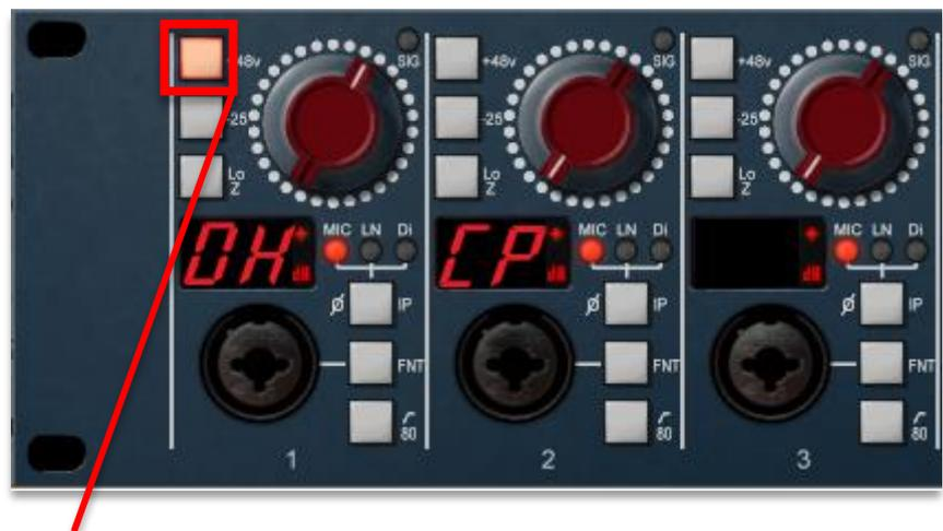
**To view the manual address menu and set a manual IP Address, press the Preamplifier Channel 1 +48v button.**
