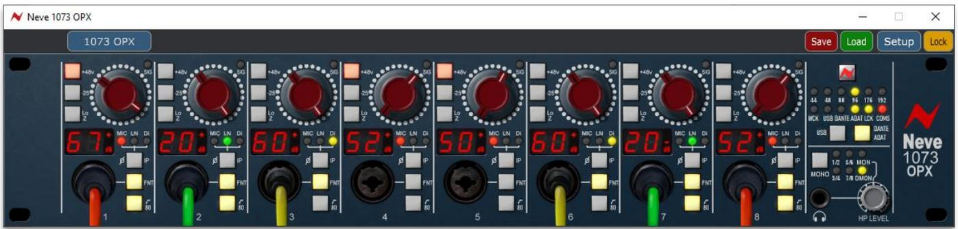
The 1073OPX proprietary Remote-control software application can be run on Mac or PC and allows users to access and operate the 1073OPX control features remotely. The unit's front panel controls including gain level, Input selection, phantom power, etc can be controlled remotely from any connected computer.
